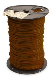
Atlas Wire MTW hook-up wire, single conductor, 12 AWG, 65-stranded, bare copper, PVC conductor insulation material, brown, 600V, 500ft spool.
