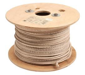
Atlas Wire MTW hook-up wire, single conductor, 10 AWG, 105-stranded, bare copper, PVC conductor insulation material, white, 600V, 500ft reel.
