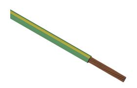
Direct Wire All-Flex flexible power cable, unshielded, MTW and THHW, single conductor, 1/0 AWG, bare copper, PVC conductor insulation material, green with yellow stripe, cut to length.
