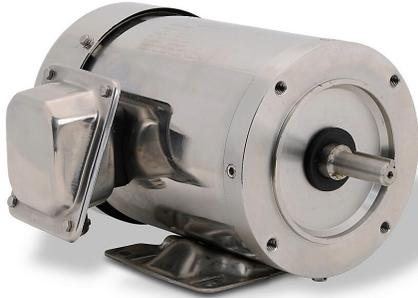
IronHorse MTS standard efficiency AC induction motor, general purpose, 3/4hp, 3-phase, 208-230/460 VAC, 3600rpm, TEFC, NEMA 56C frame, 304 stainless steel, C-face/rigid base mount. Cable gland included.
