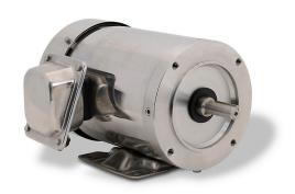
IronHorse MTS premium efficiency AC induction motor, general purpose, 3/4hp, 3-phase, 208-230/460 VAC, 1800rpm, TEFC, NEMA 56C frame, 304 stainless steel, C-face/rigid base mount. Cable gland included.
