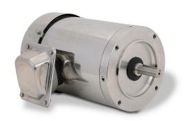
IronHorse MTS premium efficiency AC induction motor, general purpose, 3/4hp, 3-phase, 208-230/460 VAC, 1800rpm, TEFC, NEMA 56C frame, 304 stainless steel, C-face mount. Cable gland included.
