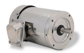
IronHorse MTS premium efficiency AC induction motor, general purpose, 3/4hp, 3-phase, 208-230/460 VAC, 1800rpm, TEFC, 56C frame, 304 stainless steel, C-face mount. Cable gland included.
