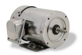
IronHorse MTS standard efficiency AC induction motor, general purpose, 1/2hp, 3-phase, 208-230/460 VAC, 3600rpm, TEFC, NEMA 56C frame, 304 stainless steel, C-face/rigid base mount. Cable gland included.
