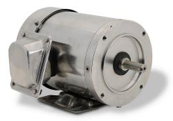
IronHorse MTS premium efficiency AC induction motor, general purpose, 1/2hp, 3-phase, 208-230/460 VAC, 1800rpm, TEFC, NEMA 56C frame, 304 stainless steel, C-face/rigid base mount. Cable gland included.
