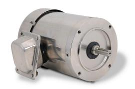
IronHorse MTS premium efficiency AC induction motor, general purpose, 1/2hp, 3-phase, 208-230/460 VAC, 1800rpm, TEFC, NEMA 56C frame, 304 stainless steel, C-face mount. Cable gland included.
