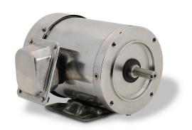
IronHorse MTS premium efficiency AC induction motor, general purpose, 1/3hp, 3-phase, 208-230/460 VAC, 1800rpm, TEFC, NEMA 56C frame, 304 stainless steel, C-face/rigid base mount. Cable gland included.
