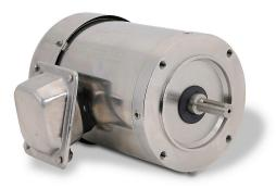
IronHorse MTS premium efficiency AC induction motor, general purpose, 1/3hp, 3-phase, 208-230/460 VAC, 1800rpm, TEFC, NEMA 56C frame, 304 stainless steel, C-face mount. Cable gland included.
