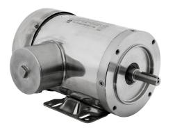
IronHorse MTS premium efficiency AC induction motor, washdown and inverter rated, 3/4hp, 3-phase, 208-230/460 VAC, 3600rpm, TEFC, NEMA 56C frame, 304 stainless steel, C-face/rigid base mount.
