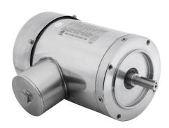
IronHorse MTS premium efficiency AC induction motor, washdown and inverter rated, 3/4hp, 3-phase, 208-230/460 VAC, 3600rpm, TEFC, 56C frame, 304 stainless steel, C-face mount.
