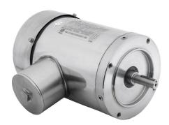
IronHorse MTS premium efficiency AC induction motor, washdown and inverter rated, 3/4hp, 3-phase, 208-230/460 VAC, 3600rpm, TEFC, NEMA 56C frame, 304 stainless steel, C-face mount.
