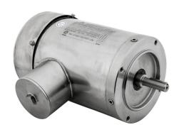
IronHorse MTS premium efficiency AC induction motor, washdown and inverter rated, 3/4hp, 3-phase, 208-230/460 VAC, 1800rpm, TEFC, 56C frame, 304 stainless steel, C-face mount.
