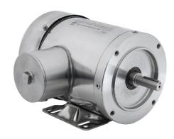
IronHorse MTS premium efficiency AC induction motor, washdown and inverter rated, 1/2hp, 3-phase, 208-230/460 VAC, 3600rpm, TEFC, NEMA 56C frame, 304 stainless steel, C-face/rigid base mount.
