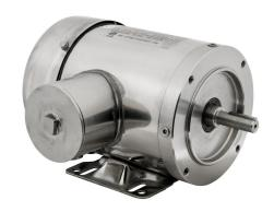
IronHorse MTS premium efficiency AC induction motor, washdown and inverter rated, 1/2hp, 3-phase, 208-230/460 VAC, 1800rpm, TEFC, NEMA 56C frame, 304 stainless steel, C-face/rigid base mount.
