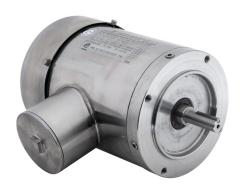
IronHorse MTS premium efficiency AC induction motor, washdown and inverter rated, 1/2hp, 3-phase, 208-230/460 VAC, 1800rpm, TEFC, NEMA 56C frame, 304 stainless steel, C-face mount.
