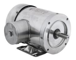
IronHorse MTS premium efficiency AC induction motor, washdown and inverter rated, 1/2hp, 3-phase, 208-230/460 VAC, 1200rpm, TEFC, NEMA 56C frame, 304 stainless steel, C-face/rigid base mount.
