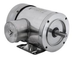
IronHorse MTS premium efficiency AC induction motor, washdown and inverter rated, 1/3hp, 3-phase, 208-230/460 VAC, 3600rpm, TEFC, NEMA 56C frame, 304 stainless steel, C-face/rigid base mount.
