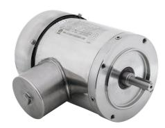
IronHorse MTS premium efficiency AC induction motor, washdown and inverter rated, 1/3hp, 3-phase, 208-230/460 VAC, 3600rpm, TEFC, NEMA 56C frame, 304 stainless steel, C-face mount.
