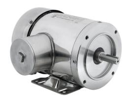
IronHorse MTS premium efficiency AC induction motor, washdown and inverter rated, 1/3hp, 3-phase, 208-230/460 VAC, 1800rpm, TEFC, NEMA 56C frame, 304 stainless steel, C-face/rigid base mount.
