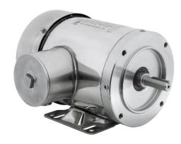
IronHorse MTS premium efficiency AC induction motor, washdown, inverter rated and hazardous location, 1/3hp, 3-phase, 208-230/460 VAC, 1800rpm, TEFC, 56C frame, 304 stainless steel, C-face/rigid base mount.
