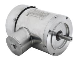
IronHorse MTS premium efficiency AC induction motor, washdown and inverter rated, 1/3hp, 3-phase, 208-230/460 VAC, 1800rpm, TEFC, NEMA 56C frame, 304 stainless steel, C-face mount.
