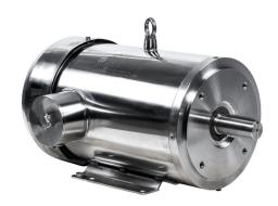
IronHorse MTS premium efficiency AC induction motor, washdown and inverter rated, 7-1/2hp, 3-phase, 208-230/460 VAC, 1800rpm, TEFC, NEMA 213TC frame, 304 stainless steel, C-face/rigid base mount.
