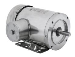
IronHorse MTS premium efficiency AC induction motor, washdown and inverter rated, 1-1/2hp, 3-phase, 208-230/460 VAC, 3600rpm, TEFC, NEMA 56C frame, 304 stainless steel, C-face/rigid base mount.
