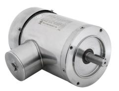
IronHorse MTS premium efficiency AC induction motor, washdown and inverter rated, 1-1/2hp, 3-phase, 208-230/460 VAC, 3600rpm, TEFC, NEMA 143TC frame, 304 stainless steel, C-face mount.
