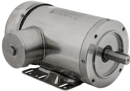
IronHorse MTS premium efficiency AC induction motor, washdown and inverter rated, 1-1/2hp, 3-phase, 208-230/460 VAC, 3600rpm, TEFC, NEMA 143TC frame, 304 stainless steel, C-face/rigid base mount.
