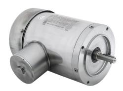
IronHorse MTS premium efficiency AC induction motor, washdown and inverter rated, 1-1/2hp, 3-phase, 208-230/460 VAC, 1800rpm, TEFC, NEMA 56C frame, 304 stainless steel, C-face mount.
