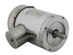
IronHorse MTS premium efficiency AC induction motor, washdown and inverter rated, 1-1/2hp, 3-phase, 208-230/460 VAC, 1800rpm, TEFC, NEMA 145TC frame, 304 stainless steel, C-face mount.
