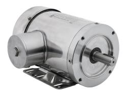
IronHorse MTS premium efficiency AC induction motor, washdown and inverter rated, 1-1/2hp, 3-phase, 208-230/460 VAC, 1800rpm, TEFC, NEMA 145TC frame, 304 stainless steel, C-face/rigid base mount.
