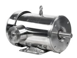
IronHorse MTS premium efficiency AC induction motor, washdown and inverter rated, 1-1/2hp, 3-phase, 208-230/460 VAC, 1200rpm, TEFC, NEMA 182TC frame, 304 stainless steel, C-face/rigid base mount.
