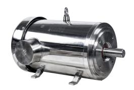
IronHorse MTS premium efficiency AC induction motor, washdown and inverter rated, 20hp, 3-phase, 208-230/460 VAC, 1800rpm, TEFC, 256TC frame, 304 stainless steel, C-face/rigid base mount.
