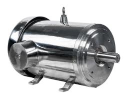
IronHorse MTS premium efficiency AC induction motor, washdown and inverter rated, 15hp, 3-phase, 208-230/460 VAC, 1800rpm, TEFC, NEMA 254TC frame, 304 stainless steel, C-face/ rigid base mount.
