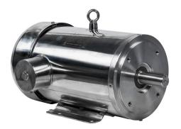
IronHorse MTS premium efficiency AC induction motor, washdown and inverter rated, 10hp, 3-phase, 208-230/460 VAC, 1800rpm, TEFC, NEMA 215TC frame, 304 stainless steel, C-face/ rigid base mount.
