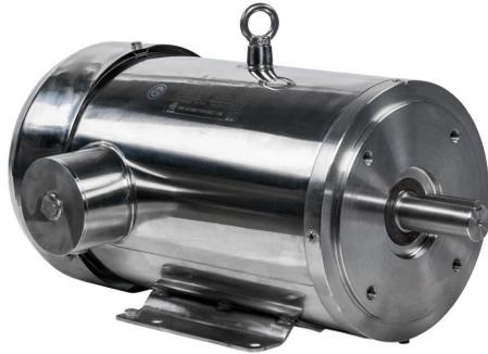
IronHorse MTS premium efficiency AC induction motor, washdown and inverter rated, 10hp, 3-phase, 208-230/460 VAC, 1800rpm, TEFC, NEMA 215TC frame, 304 stainless steel, C-face/ rigid base mount.
