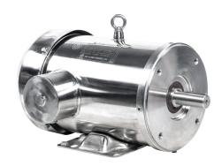
IronHorse MTS premium efficiency AC induction motor, washdown and inverter rated, 5hp, 3-phase, 208-230/460 VAC, 3600rpm, TEFC, 184TC frame, 304 stainless steel, C-face/rigid base mount.
