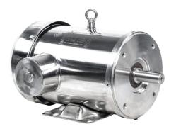
IronHorse MTS premium efficiency AC induction motor, washdown and inverter rated, 5hp, 3-phase, 208-230/460 VAC, 3600rpm, TEFC, NEMA 184TC frame, 304 stainless steel, C-face/ rigid base mount.
