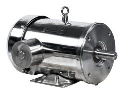
IronHorse MTS premium efficiency AC induction motor, washdown and inverter rated, 5hp, 3-phase, 208-230/460 VAC, 1800rpm, TEFC, NEMA 184TC frame, 304 stainless steel, C-face/ rigid base mount.
