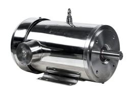
IronHorse MTS premium efficiency AC induction motor, washdown and inverter rated, 5hp, 3-phase, 208-230/460 VAC, 1200rpm, TEFC, 215TC frame, 304 stainless steel, C-face/rigid base mount.
