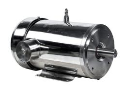
IronHorse MTS premium efficiency AC induction motor, washdown and inverter rated, 5hp, 3-phase, 208-230/460 VAC, 1200rpm, TEFC, NEMA 215TC frame, 304 stainless steel, C-face/rigid base mount.
