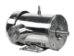
IronHorse MTS premium efficiency AC induction motor, washdown and inverter rated, 3hp, 3-phase, 208-230/460 VAC, 3600rpm, TEFC, NEMA 182TC frame, 304 stainless steel, C-face/rigid base mount.
