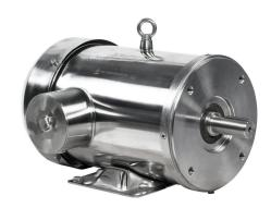
IronHorse MTS premium efficiency AC induction motor, washdown and inverter rated, 3hp, 3-phase, 208-230/460 VAC, 1800rpm, TEFC, NEMA 182TC frame, 304 stainless steel, C-face/rigid base mount.
