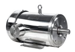
IronHorse MTS premium efficiency AC induction motor, washdown and inverter rated, 3hp, 3-phase, 208-230/460 VAC, 1200rpm, TEFC, 213TC frame, 304 stainless steel, C-face/rigid base mount.
