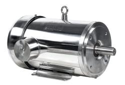
IronHorse MTS premium efficiency AC induction motor, washdown and inverter rated, 3hp, 3-phase, 208-230/460 VAC, 1200rpm, TEFC, NEMA 213TC frame, 304 stainless steel, C-face/ rigid base mount.
