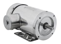
IronHorse MTS premium efficiency AC induction motor, washdown and inverter rated, 2hp, 3-phase, 208-230/460 VAC, 3600rpm, TEFC, NEMA 56C frame, 304 stainless steel, C-face/rigid base mount.
