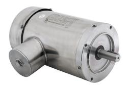
IronHorse MTS premium efficiency AC induction motor, washdown and inverter rated, 2hp, 3-phase, 208-230/460 VAC, 3600rpm, TEFC, NEMA 145TC frame, 304 stainless steel, C-face mount.
