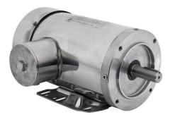
IronHorse MTS premium efficiency AC induction motor, washdown and inverter rated, 2hp, 3-phase, 208-230/460 VAC, 3600rpm, TEFC, NEMA 145TC frame, 304 stainless steel, C-face/ rigid base mount.
