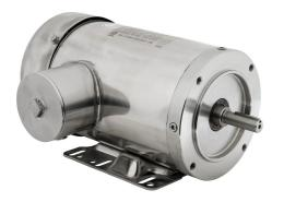
IronHorse MTS premium efficiency AC induction motor, washdown and inverter rated, 2hp, 3-phase, 208-230/460 VAC, 1800rpm, TEFC, NEMA 56C frame, 304 stainless steel, C-face/rigid base mount.
