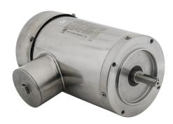
IronHorse MTS premium efficiency AC induction motor, washdown and inverter rated, 2hp, 3-phase, 208-230/460 VAC, 1800rpm, TEFC, NEMA 56C frame, 304 stainless steel, C-face mount.
