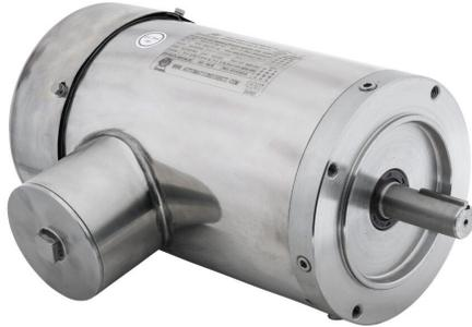
IronHorse MTS premium efficiency AC induction motor, washdown and inverter rated, 2hp, 3-phase, 208-230/460 VAC, 1800rpm, TEFC, NEMA 145TC frame, 304 stainless steel, C-face mount.
