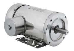
IronHorse MTS premium efficiency AC induction motor, washdown and inverter rated, 2hp, 3-phase, 208-230/460 VAC, 1800rpm, TEFC, NEMA 145TC frame, 304 stainless steel, C-face/ rigid base mount.
