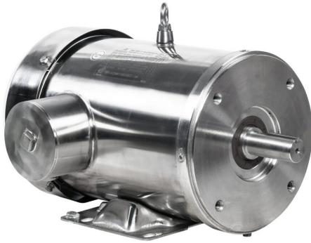
IronHorse MTS premium efficiency AC induction motor, washdown and inverter rated, 2hp, 3-phase, 208-230/460 VAC, 1200rpm, TEFC, NEMA 184TC frame, 304 stainless steel, C-face/ rigid base mount.
