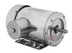
IronHorse MTS premium efficiency AC induction motor, washdown and inverter rated, 1hp, 3-phase, 208-230/460 VAC, 3600rpm, TEFC, 56C frame, 304 stainless steel, C-face/rigid base mount.
