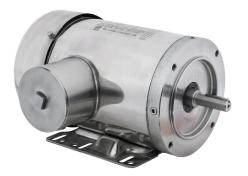
IronHorse MTS premium efficiency AC induction motor, washdown and inverter rated, 1hp, 3-phase, 208-230/460 VAC, 3600rpm, TEFC, NEMA 56C frame, 304 stainless steel, C-face/rigid base mount.
