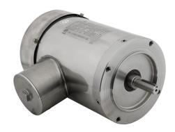
IronHorse MTS premium efficiency AC induction motor, washdown and inverter rated, 1hp, 3-phase, 208-230/460 VAC, 3600rpm, TEFC, NEMA 56C frame, 304 stainless steel, C-face mount.
