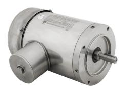
IronHorse MTS premium efficiency AC induction motor, washdown and inverter rated, 1hp, 3-phase, 208-230/460 VAC, 1800rpm, TEFC, NEMA 56C frame, 304 stainless steel, C-face mount.
